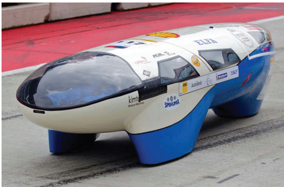
Figure 1 | Agelis ecocar built at Royal Institute of Technology KTH in Stockholm, Sweden managed to run for 481 km at 1 L of gasoline during Shell Eco Marathon 2010. Critical engine components had antifriction coatings made by Applied Nano Surfaces, and a fuel economy engine oil produced by Elektrion s.a. was used.
